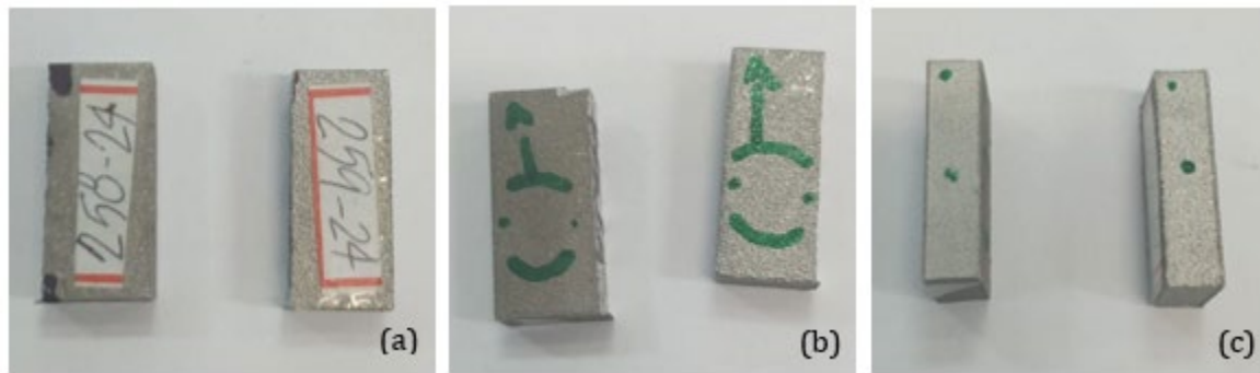
Figure 1. AA5050 samples (left: AC30 shot; right: AC50 shot), where: a – labeled samples; b – longitudinal direction marking; c – transverse (90°) direction marking.
