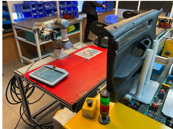
Figure 7. Door on the production line together with the vision system used and the robot.
