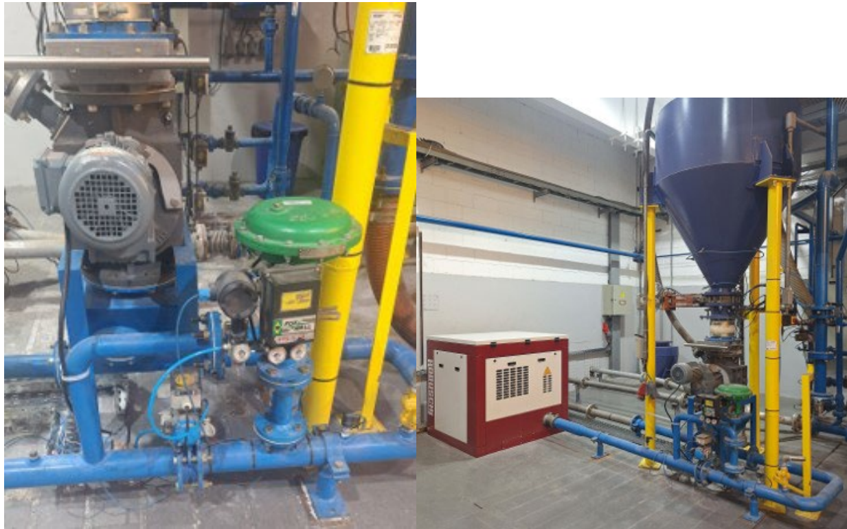
Figure 3A and 3 B- Research apparatus and set up under test showing Rotary Valve, Blower-Motor , Air Dosing Valve and surrounding piping (by Authors)
