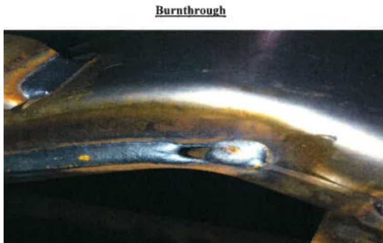
Figure 8. Burn through defect in auto parts manufacturing
