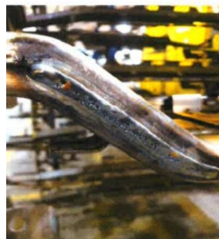
Figure 6. Porosity defects of welds in auto parts manufacturing
