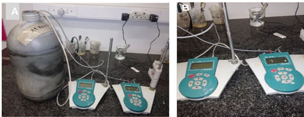
Figure 4. The leaching apparatus: (A) Leaching kinetics set-up, including the system's temperature, time, and pH control; (B) An experimental set-up of a typical duration monitor of the leaching conditions.
