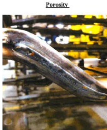
Figure 7. Porosity defects of welds in auto parts manufacturing
