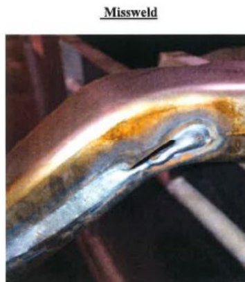
Figure 8. Misweld defects in Auto parts manufacturing
