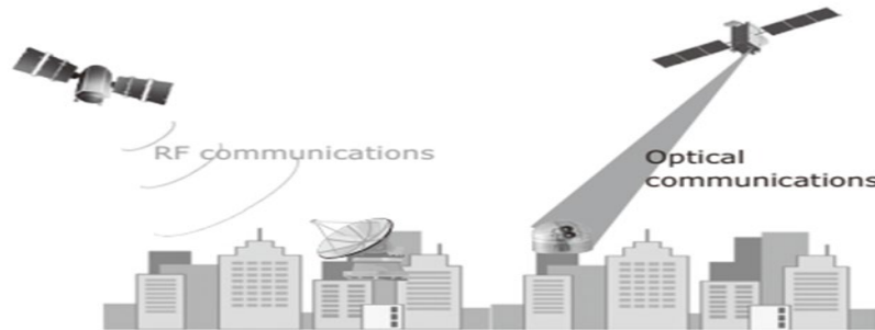
Figure 1. Image of difference in beams between RF and Optical communication
