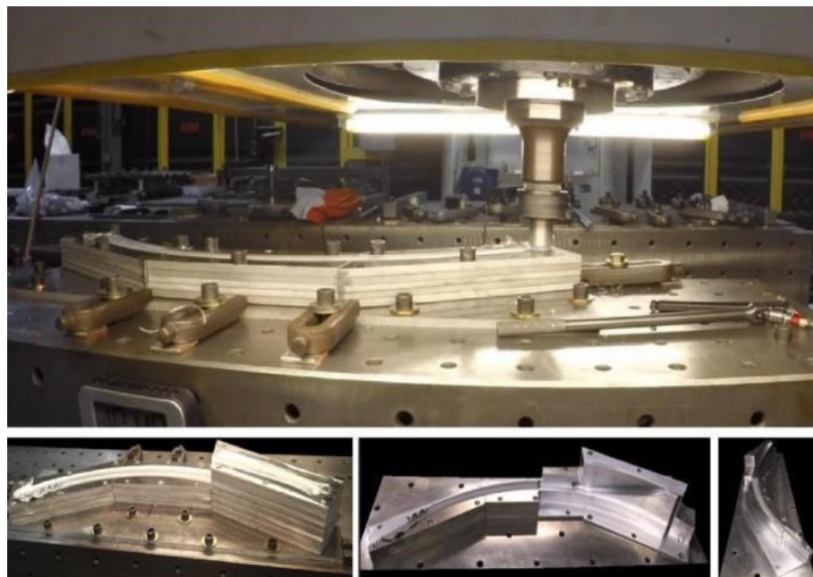
Figure 2. The experimental setup and intricate component created using FSAM by the Edison Welding Institute (EWI) (Cruz, 2022)
