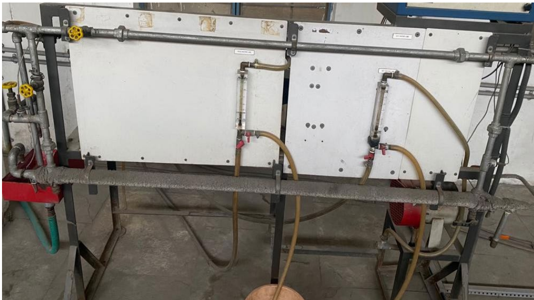
Figure 1. Experimental setup of Concentric tube Heat Exchanger
