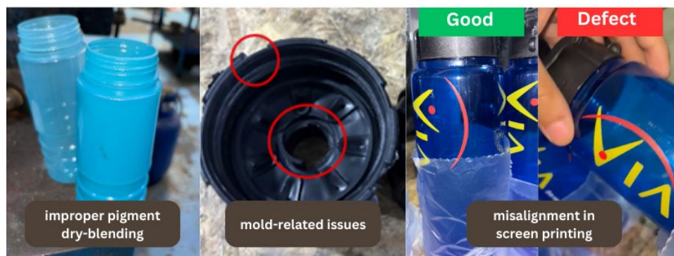
Figure 2. Principal defects type
