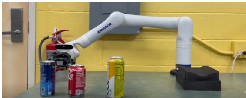
Figure 2. Experimental setup showing the Kinova Gen3 collaborative robot and predefined object locations used for color-based pick-and-place trials
