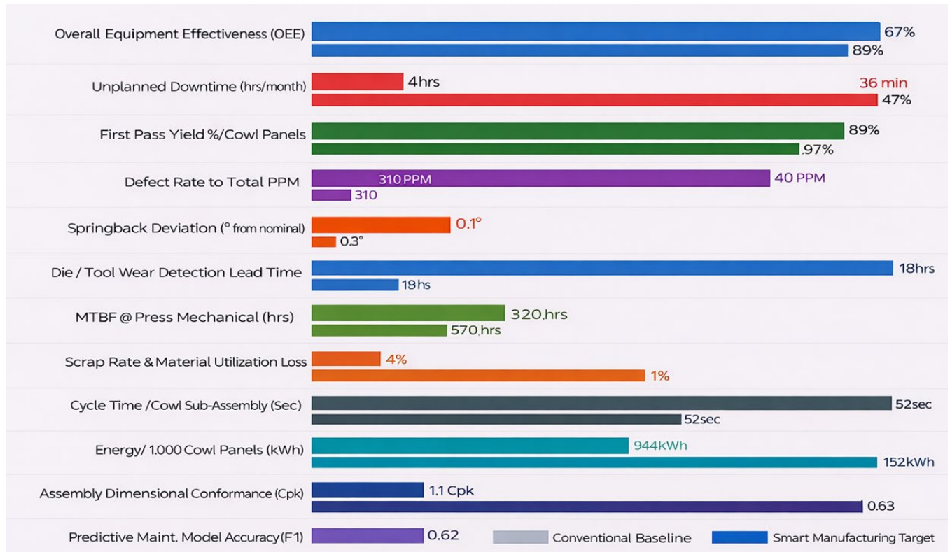
Figure 6. 12-Metric KPI Profile — Conventional vs. Smart Cowl Stamping Manufacturing
