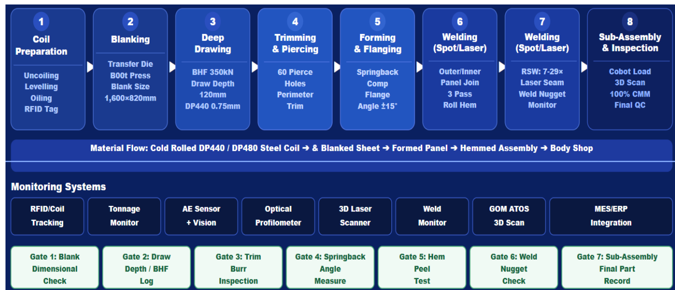
Figure 1. Cowl Panel Assembly — Stamped Parts Production Process Flow
