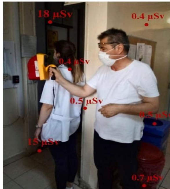
Figure 2. Measuring emission of radiation to the environment during X-ray imaging (Source: Yıldız et al. 2022)
