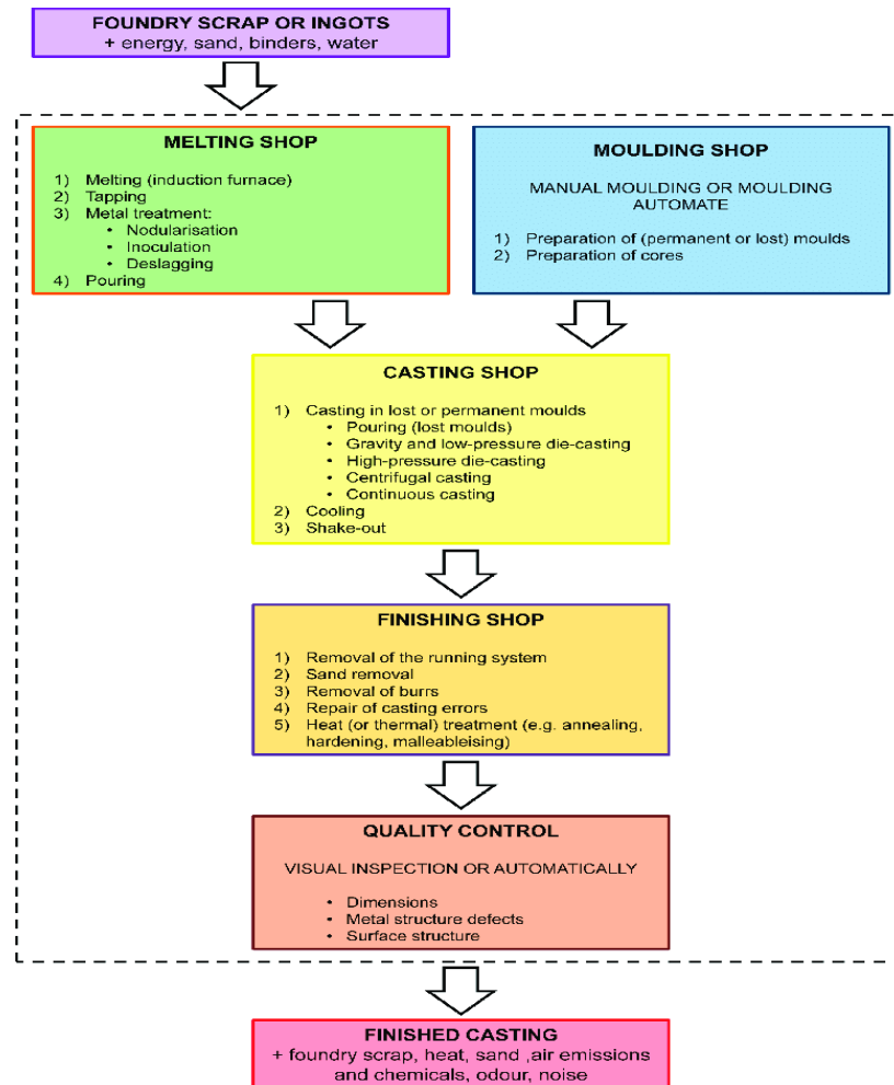
Figure 2. (a) Die casting process flow chart (Stefana, et al., 2019)
