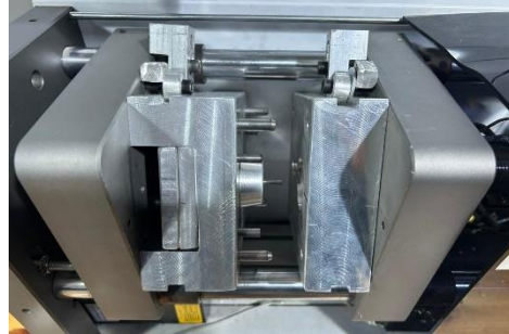
Figure 15. Mold mounted on the machine
