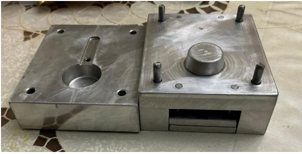
Figure 14. Finished mold (core and cavity)
