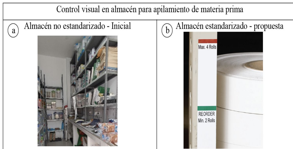
Figure 7. Visual control in the warehouse for raw material stacking
