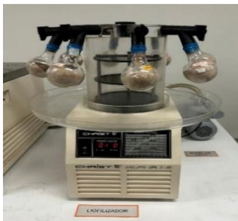
Figure 3. Ungurahui in freeze-drying machine
