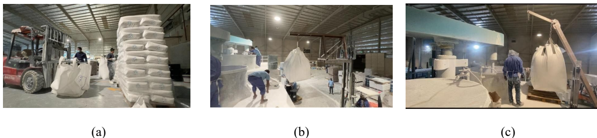
Figure 4. Alternative one: (a) large bag and the materials are transferred to the work area, (b) the forklift is raising the bags using a hook, and (c) pouring the bags containing the materials into the tank involves cutting the ends of the bags.
