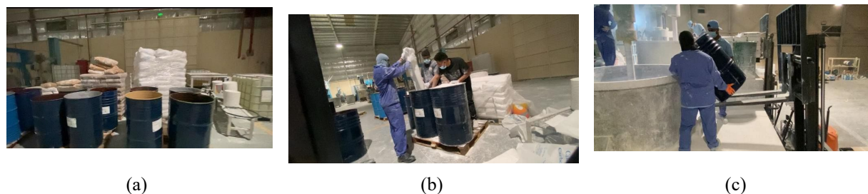
Figure 5. Alternative two: (a) the drums and materials are transferred to the work area, (b) filling the drums with all the materials in a specific arrangement, and (c) pouring the drums that contain the materials into the tank.
