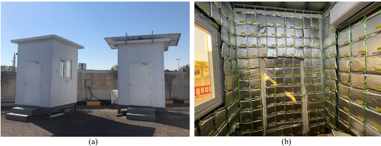
Figure 1. The experimental setup with two identical portable cabins (a), the left cabin is equipped with PCM slabs on all interior walls and the ceiling (b), while the right cabin serves as control.
