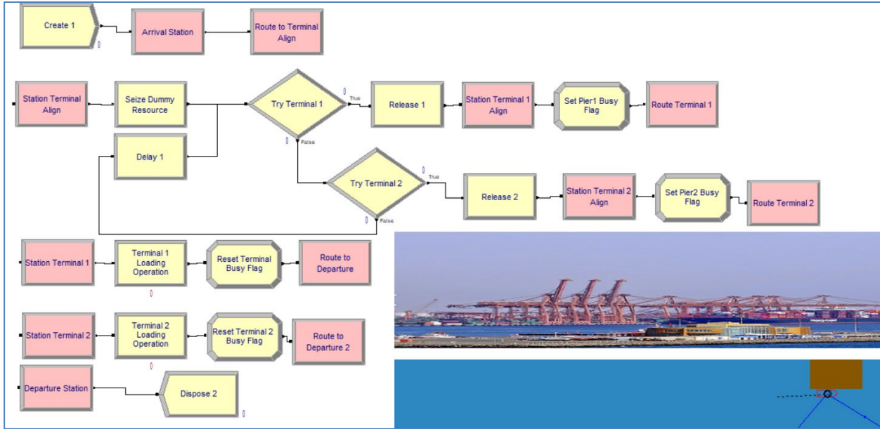
Figure 9. Logic for Container vessels flow at Jeddah Islamic Port (SAJED)
