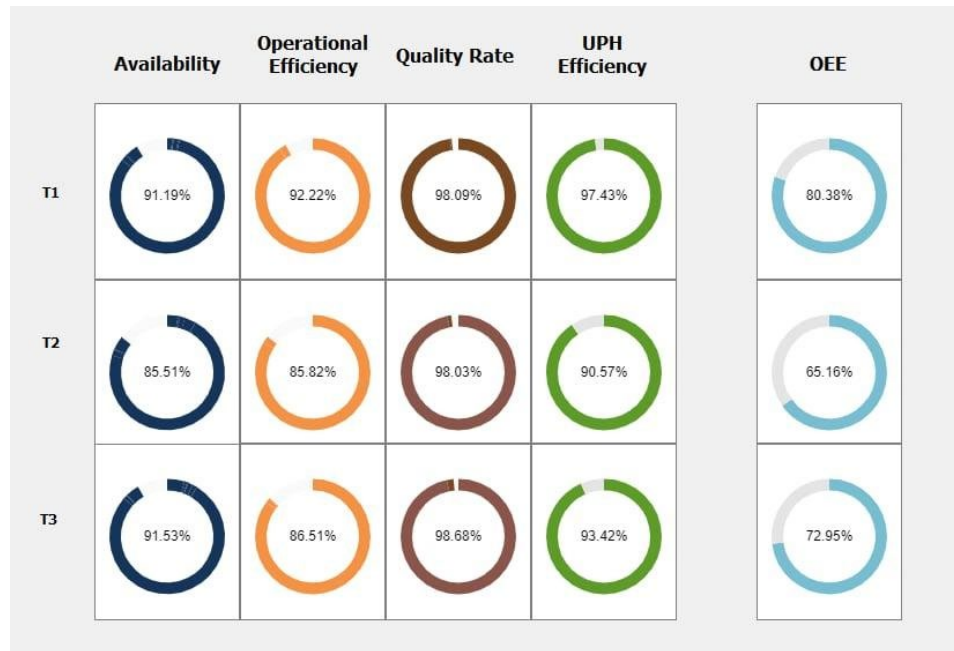
Figure 3. Dashboard showing the OEE and its components for each machine temperature
