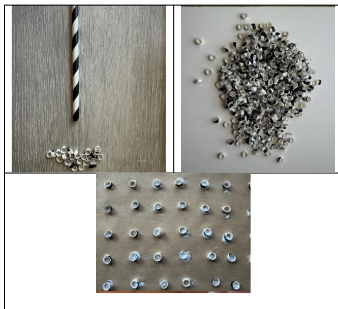
Figure 2. Alternative to bubble wrap sheet – an experiment of firm rings placed at a uniform distance on a recycled paper.
