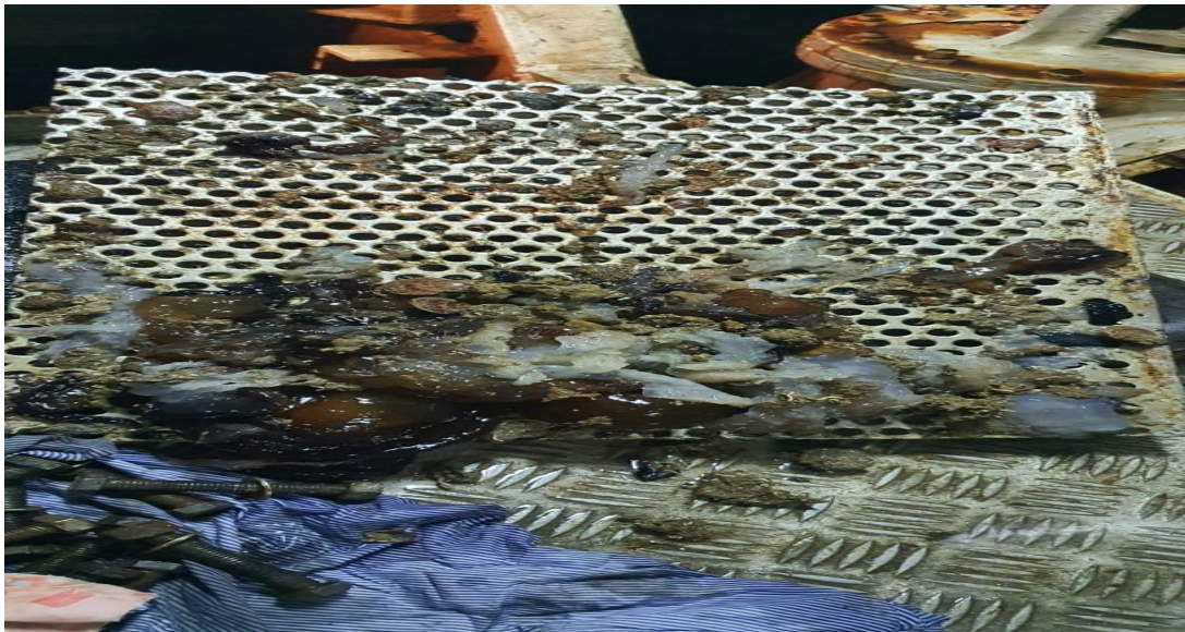
Figure 3. Effect of Sea Growth in Condenser Inlet Sea Chest Strainer.
