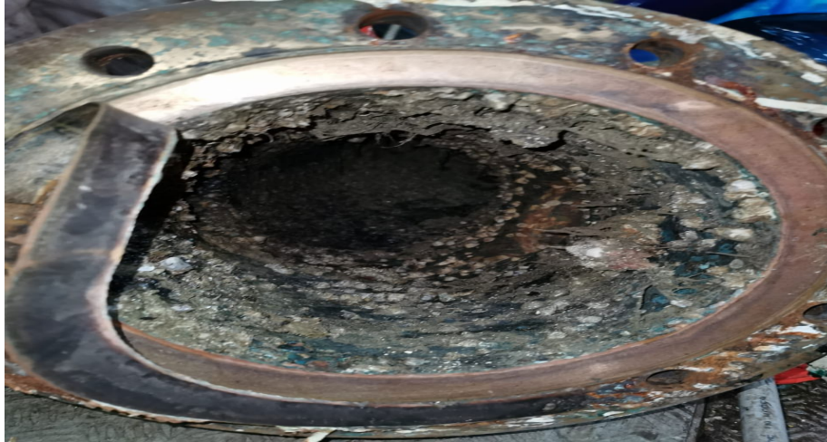
Figure 6. Effect of Biofouling in SW Cooling Line.
