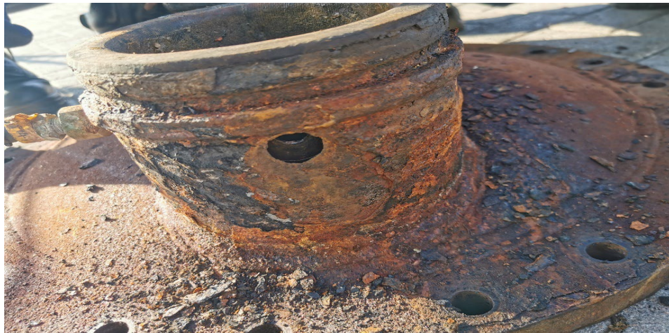
Figure 5. Effect of Corrosion in Condenser Cover.
