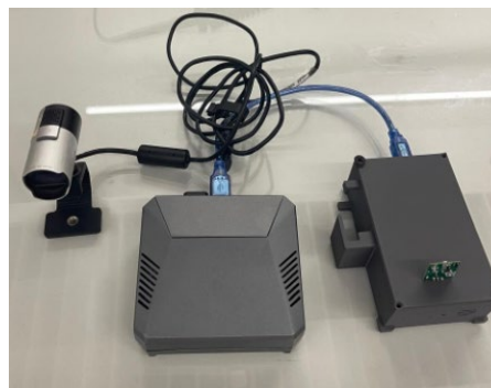
Figure 5. Transmitter module with Raspberry Pi and nRF24L01.
