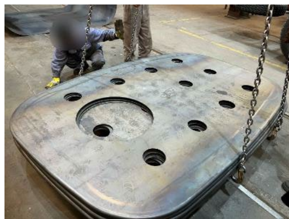
Figure 7: the oil tanker benchmark with built in baffles, Mula company Kuwait.
