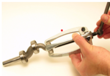
Figure. 5 One step of paper Based Instruction for replacing the grooved ball bearing
