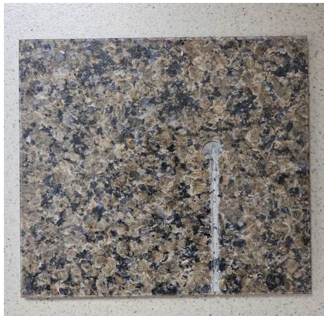
Figure 3. Photo of Sample B (15×15×1cm) obtained from Najran Granite Factory. This sample was used to calculate the thermal resistance ( R=2.96 \text{ m}^2\cdot\text{K}/\text{W} ).
