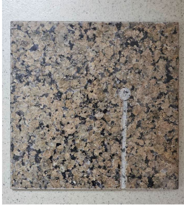
Figure 4. Photo of Sample C (15×15×1cm) obtained from Najran Granite Factory. This sample was used to calculate the thermal resistance ( R=2.11 \text{ m}^2 \cdot \text{K/W} ).
