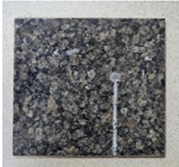
Figure 2. Photo of Sample A (15×15×1cm) obtained from Najran Granite Factory. This sample was used to calculate the thermal resistance ( R=1.08 \text{ m}^2\cdot\text{K}/\text{W} ).
