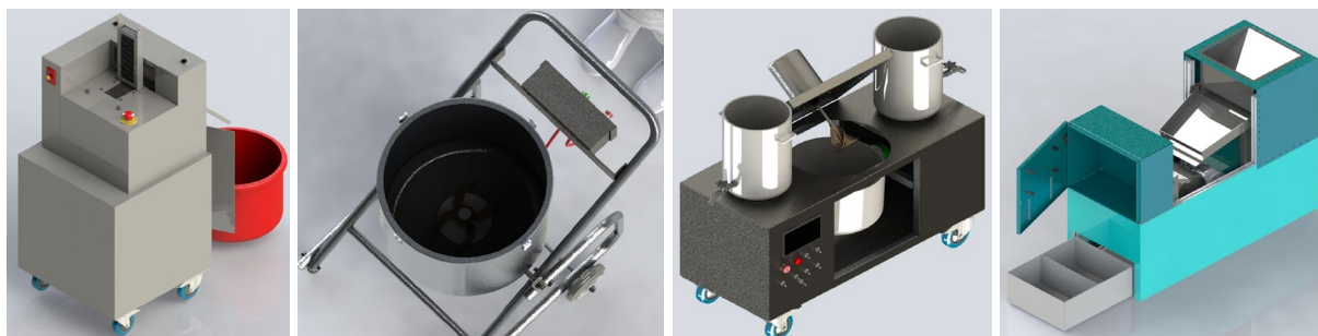
Figure 6. 3D models for each machine in the integrated system (a) de-blistering, (b) shredder, (c) chemical separation, and (d) electrostatic separation
