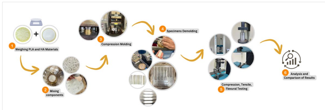
Figure 1. Experimental procedure for the fabrication and mechanical characterisation of PLA/nHA composites.
