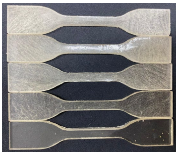
Figure 2. Dispersion of HA particles at various loadings of 0.25wt.%, 0.5wt.%, 1 wt.%, and 2 wt.%.
