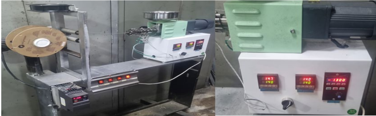
Figure 3. Extrusion and winding of PLA- pecan shell filaments
