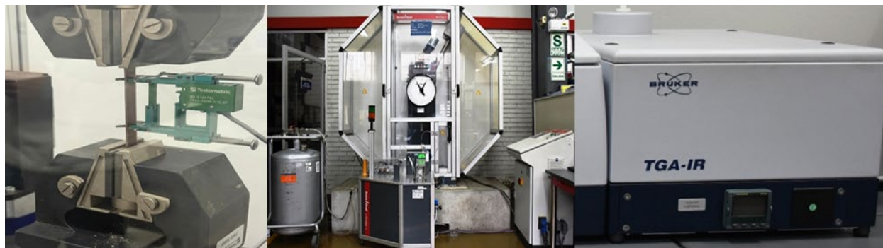
Figure 6. Equipment used for tensile, impact, and TGA testing respectively
