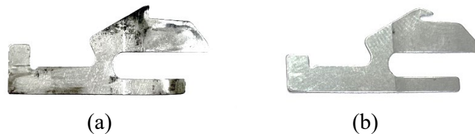
Figure 11. Sinker Condition in the Selected Machine: (a) Worn sinker, (b) New Sinker.
