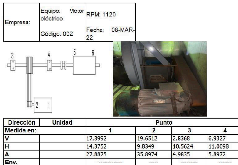
Figure 4. Vibrational Analysis for Preventive Maintenance of Electric Motor Code 002
