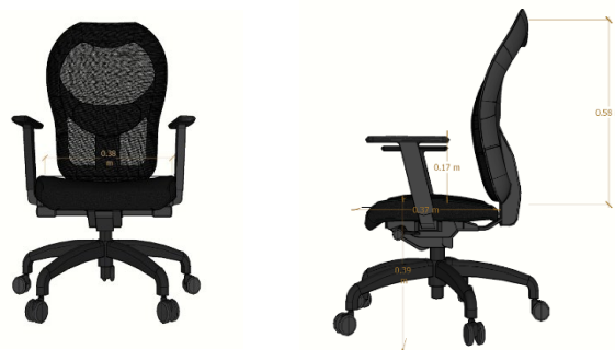
Figure 2. 3D Perspective of Proposed Ergonomic Chair Based on The Anthropometric Data of Nurses
